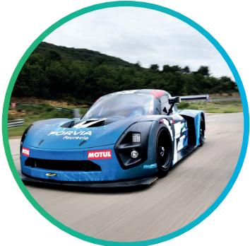
**Foenix H2, a GT racing car powered by a hydrogen combustion engine**
